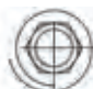
Only 3/4 Turn from Finger Tight is necessary to seal and will result in additional remakes of the fitting
