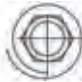
Only 3/4 Turn from Finger Tight is necessary to seal and will result in additional remakes of the fitting
