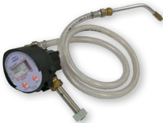
Art.no. 2824 Electronic flow meter art. no. 2429 (see page 64!) with connection adapter for manual pumps, 1 m - outlet hose and rigid outlet with automatic anti-drip nozzle.
