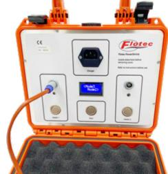
first "Pre-Heat" the Clamps and then commence the "Fix-Heat" once the PowerGrip position has been checked and confirmed.
